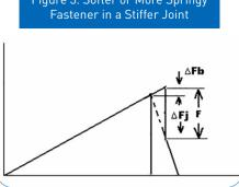
If the bolt is less stiff, with respect to the joint, the bolt will experience a smaller percentage of the external load, which depends upon the stiffness ratio of the bolt and joint. This helps in
