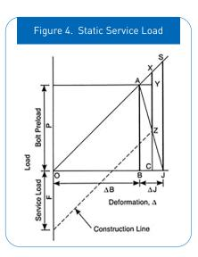
determining what type and size of bolt to use in the joint. The stiffness ratio can also help determine preloads, loss due to embedment and bolt failure.
